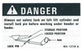
Raise feeder to maximum up position and lower safety stop over the piston rod of the header lift cylinder and pin in place. Then lower feeder to lock stop in place.
