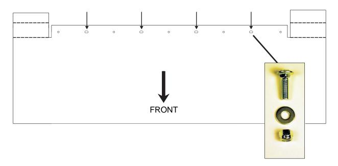
STEP 9 Using the remaining pre-drilled holes as a guide, drill thru the floor of the header with the 9/32" drill bit supplied.
